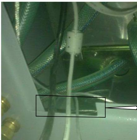
Make sure power cable, data cable and sensor line wear out from the gap of back panel.
